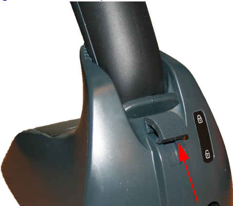
Figure 2. Lever in locked position
